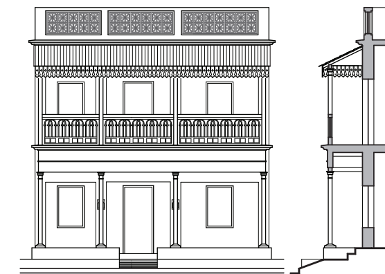
Elevation and section of a flat roofed thalvaram with balcony above
